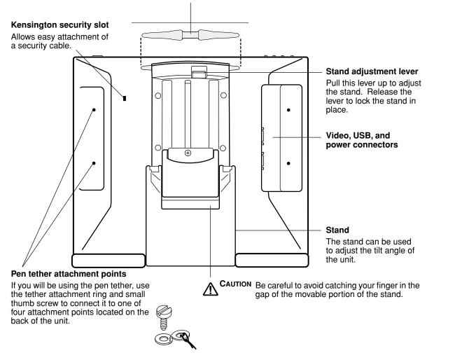
**Important:** Be sure to adjust the stand to the low tilt position before packaging the DTF-521/PL-521. If you do not close the stand, the notched mechanism may be damaged during transportation and storage. Do not lift the unit by the stand; this may damage the stand mechanism. When lifting or moving the pen display, always do so by grasping the main body casing.
